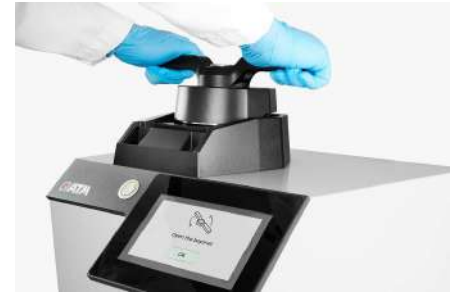
3. Lock the bayonet quick-release closure.
