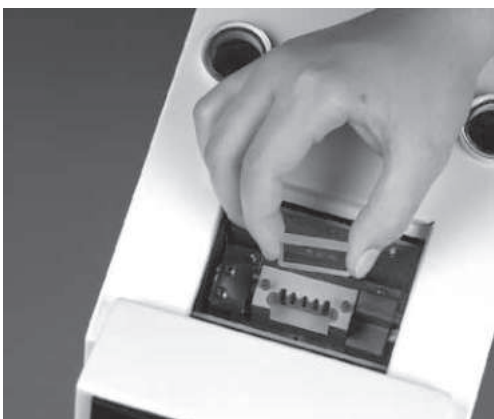
Figure 5: Mounting the glass panel
