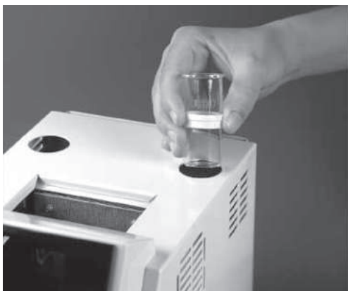
Figure 4: Mounting the glass sample holder
