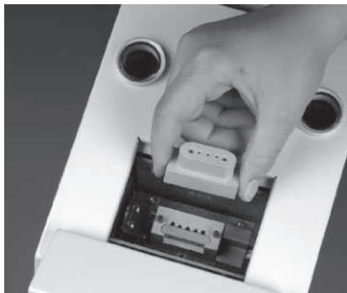
Figure 6: Inserting the upper ceramic part
