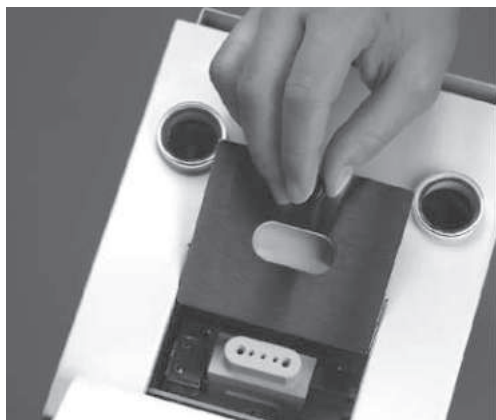
Figure 7: Fitting the metal cover
